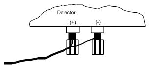
To analog input A, B, C, or D of the system interface
