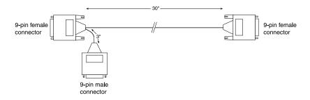
Refer to the diagram below to connect the 506C to another Gilson device using a GSIOC cable.
