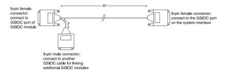
With additional GSIOC cables, you can connect as many as 32 slave devices. To connect additional GSIOC cables, connect the male connector to the next cable's female connector (use the female connector that's not joined to the male connector). Then connect the remaining female connector to the GSIOC port of the device.
