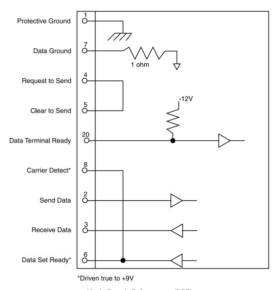
25-pin Female D-Connector (DCE)
