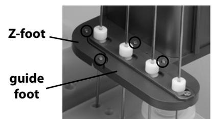
**guide foot installed on Z-foot**
