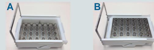
Custom magnetic bead separator used in the automated procedure. The handle of the device can be actuated by the liquid handler to move the magnets from the disengaged lower position (A) to the engaged upper position (B). When engaged, each magnet is in proximity to 4 wells of a 96 well plate.
