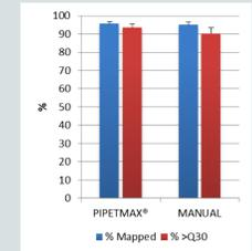
The percentage of mapped reads and the quality scores (% >Q30) were averaged across twelve replicate libraries prepared either with automated or manual pipetting. The automated methods provided reproducible liquid handling, resulting in smaller standard deviations and lower variance between replicates.
