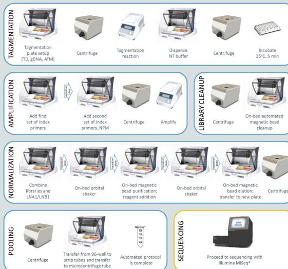
Each blue rounded rectangle represents one PIPETMAX script, each of which corresponds to a portion of the Nextera XT System workflow. Some user intervention may be required to reposition labware or centrifuge a microplate between liquid handling steps.
