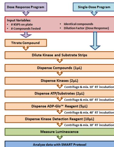
**Figure 3. The user selects the desired profiling protocol to run and reagents are added to the bed of the PIPETMAX®. The PIPETMAX® performs all liquid handling steps as shown here. Centrifugation, mixing, and detection are performed off-line, while room temperature reaction incubations are performed on the bed of the instrument.**
