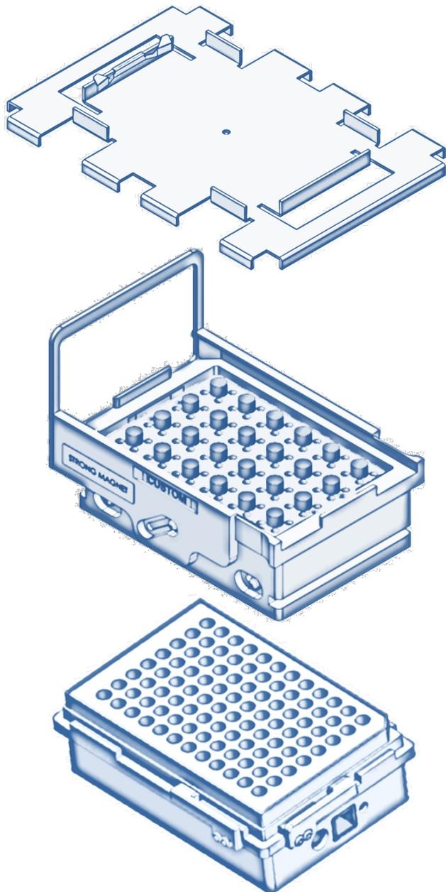
1. The portrait orientation rack (SPL-2141C-HDW) is used in the amplification script. This rack allows the user to manually rotate the reaction plate 90°, which enables multichannel addition of the index primers.
